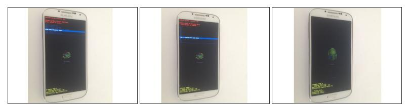
• Release them when the Android System Recovery screen appears. Use Volume Up/Down keys for navigation and Power On key for OK. Choose "wipe cache partition", "Yes -- delete all user data", "reboot system now".
