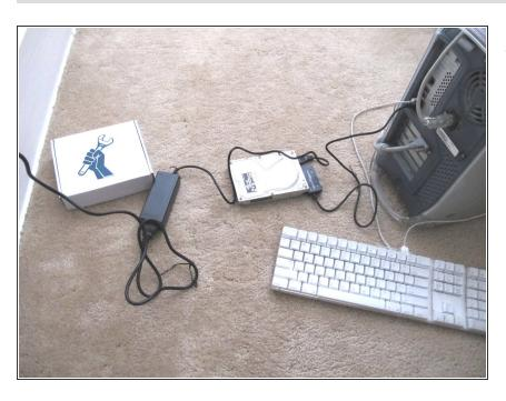
Problem: How to move HD data from an old 486 computer with no modern data transfer ports to a newer computer (i.e. Mac G4 tower). Solution: Remove hard drive from old PC and connect it to a drive adapter which can connect to the computer to which you want to move the data.
