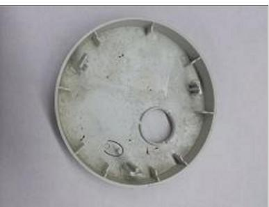
• Use a screwdriver to pry open the plastic enclosure. It might be easier to push the buzzer through the hole, if you need extra leverage.
