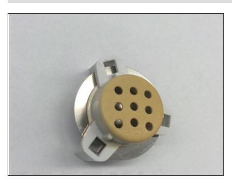
The buzzer is unhooked from the PCB board, by hands.
