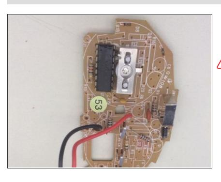
↑ The metal cap is removed to reveal a, MC145017, driver chip and americium sensor. Do not remove americium from the sensor!
