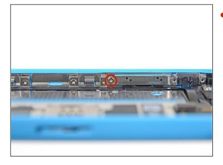
Remove the 1.6 mm Phillips #000 screw securing the volume rocker bracket to the side wall.
