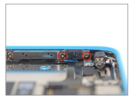
• Remove the two 1.6 mm Phillips #000 screws from the hold switch bracket.
