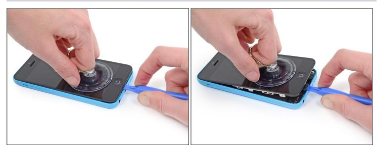
(i) Make sure the suction cup is firmly attached to the front panel assembly.
