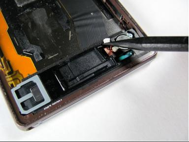
Disconnect the vibrate motor flux cable by using the spudger to gently pop it up.
