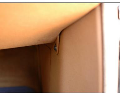
Then remove any metal screws, and any plastic trim screws, at the sides of the kick panel below the dash.
