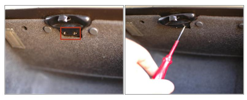
• Remove the two phillips screws in the glove box door catch, then remove it.
