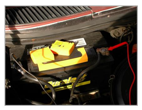
Connect the tester leads on your meter to the terminals on your battery. The red lead goes on the positive (+) terminal on your battery, and the black lead goes on the negative (-) terminal.
