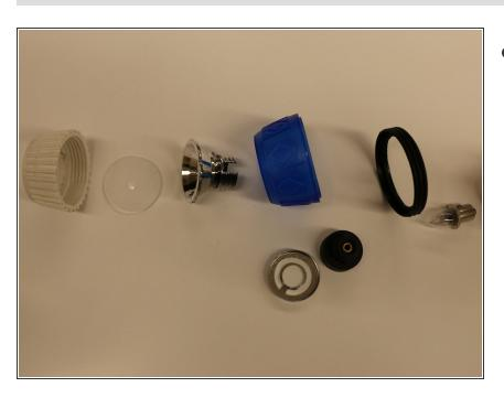
The complete light bulb component disassembly.
