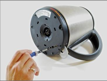
• Remove the five 3/8" screws from the base of the kettle using a Phillips #1 screwdriver.
