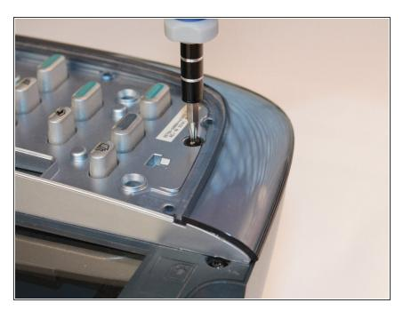
Use a T9 torx screwdriver to remove the 0.9 cm screw.
