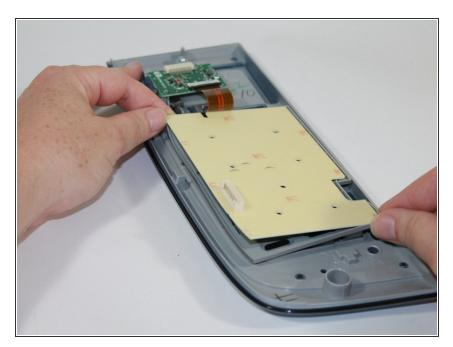
Gently lift the button panel off the plastic backing with rubber button mat.
