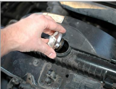
With the hood on your car up, begin by opening the radiator cap to allow the radiator to drain more efficiently.
