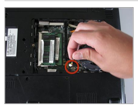
Unplug the shown cable attaching the cooling fan to the computer.
