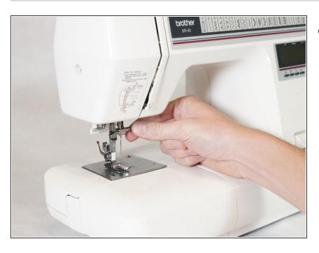
Loosen the needle by turning the knob counterclockwise.
