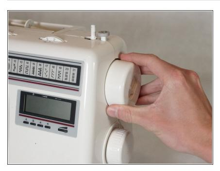
Adjust the needle to the top of its stroke using the hand wheel.
