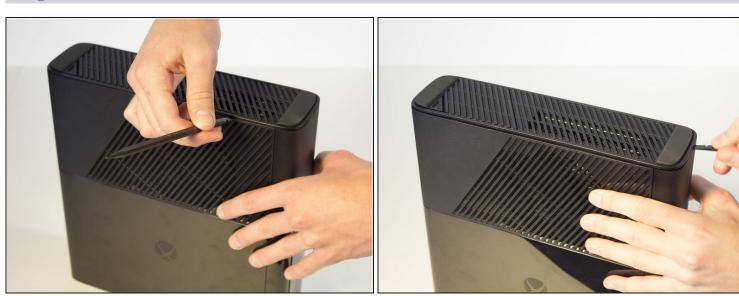
• Slide the spudger along the crevice to separate the grated face and the top body.
