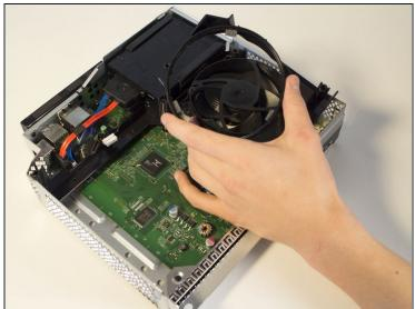
• Flip the Xbox over and take out the heat sink plastic shield.
