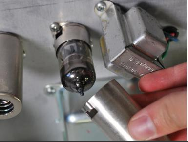
Remove the metal casing by gently pressing up against the case and twisting to the right.
