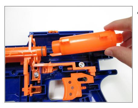
Pull the plunger towards the rear of the rifle to remove it.
