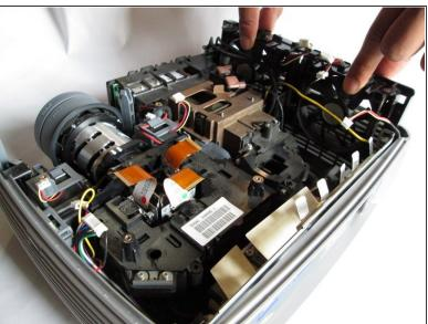
Once the main board has been removed, carefully lift the fans upward. Make sure no cables are tangled in the process.
