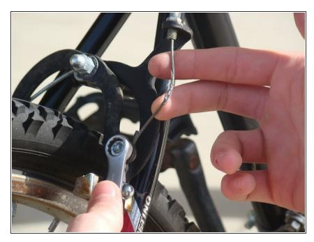
Loosen the bolt that clamps the brake cable on the brake caliper with the 10mm open-end wrench.
