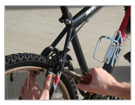
Pull the brake cable until proper tension is acquired and the cable shows resistance.
