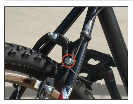
Re-tighten the clamping nut.
