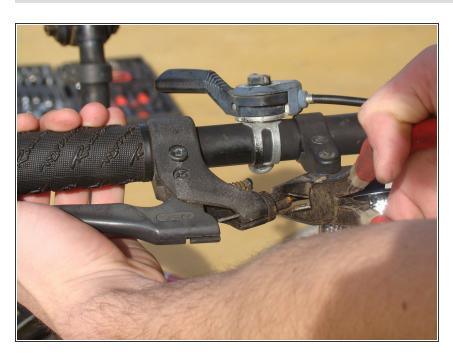
For more precise adjustment of the brake cable tension, use pliers to tighten the barrel nut at the opposite ends of the handlebars on the brake levers.
