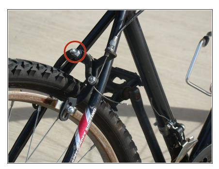
If necessary, adjust the positioning of the caliper arms by loosening the dome nut at the pivot point and manually shifting the arms in the desired direction.
