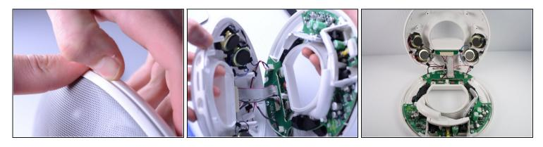
• Open the device along its seam.
