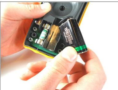
Mhen doing this next step, make sure to remove the battery slowly, so you don't damage the wires connecting the battery to the device.
