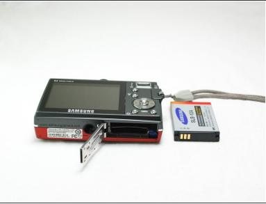
Open the battery cover that's located on the bottom right side of the camera and carefully remove the battery.
