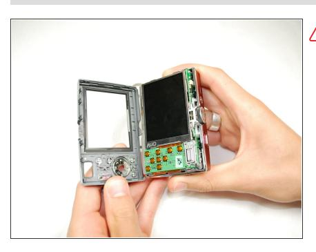
Carefully pull off the back cover, parts behind the back of the case might fall out.
