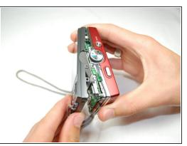
Slide your fingernail or a plastic spudger in the groove from the bottom to the top right side of the camera.
