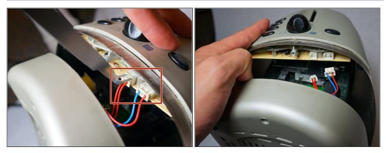
• Disconnect the cable clips from the circuit board using the <u>tweezers</u> to free the outer metal shell from the plastic base.
