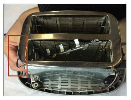
Push down on the opposite side of the bread lift shelf to expose the metal flaps.
