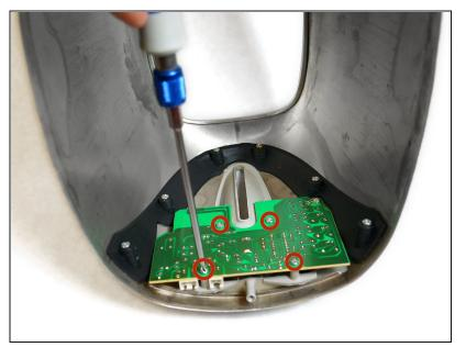
Using a #1 phillips head screwdriver, remove the four 1cm philips head screws holding the circuit board to the inside of the toaster shell.
