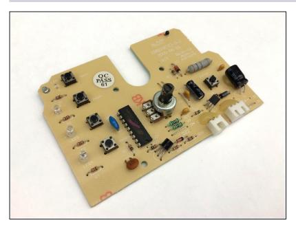
Inspect the circuit board for any burnt or otherwise damaged components. Be sure to carefully identify the damaged components that need replacement. For help identifying resistor values look at wikipedia's electronic color code article.
