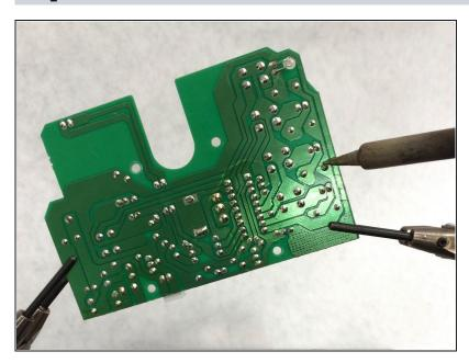
Use the soldering kit to unsolder the damaged component. For soldering Instructions look at the <u>iFixit</u> <u>Soldering Guide</u>.
