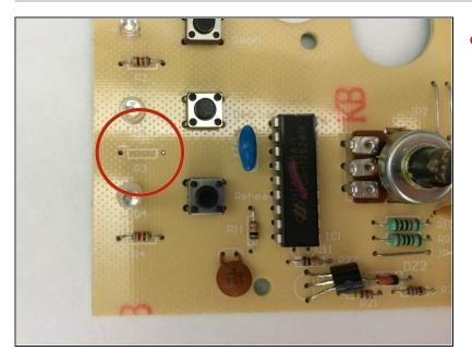
• Once the damaged component has been unsoldered from the circuit board, remove it.
