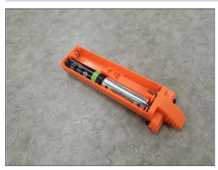
i When installing new batteries, ensure that their polarities are facing the correct directions. Follow the inscriptions on the bottom of the battery tray, or place the flat side of each battery against the spring.
