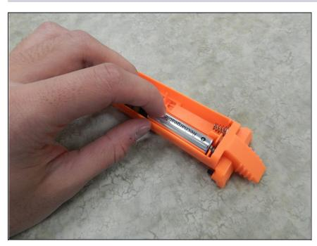
Apply downwards pressure on the battery you're trying to remove in the direction of the spring.
