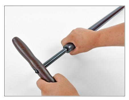
Lift the pump handle until the top cap is expsoed
