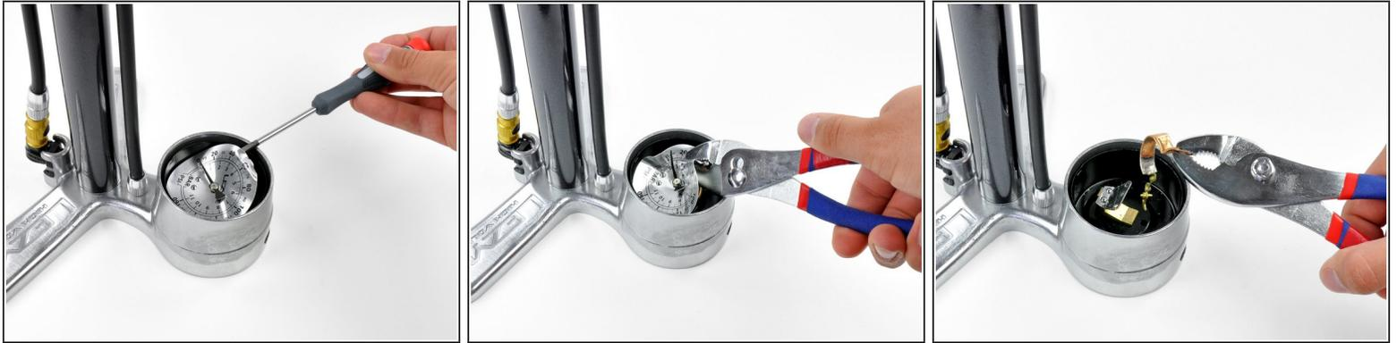
**i** No parts from the old gauge will be re-used, so there is no need to attempt to preserve the parts. However, be careful not to damage the gauge housing.
