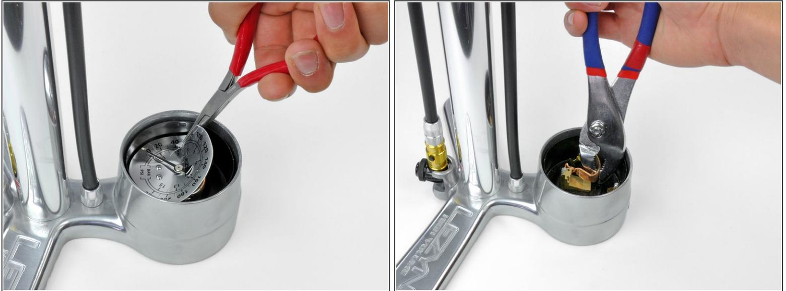
**i** No parts from the old gauge will be re-used, so there is no need to attempt to preserve the parts. However, be careful not to damage the gauge housing.
