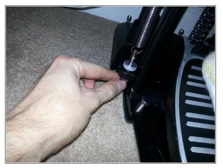
Tighten and loosen the nuts on the bottom of the springs until both pedals have an even, comfortable tension.
