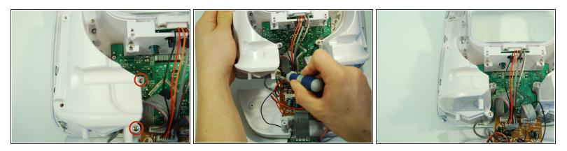
Use a Phillips #1 screwdriver to unscrew the two 8 mm screws on the speaker housing.
