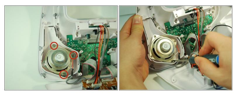
• Unscrew the three 8 mm circled screws that are holding the speaker to the plastic casing.
