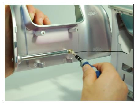
Use a Phillips #1 screwdriver to detach the wire from the back panel by removing the 8 mm screw connecting the wire to the antenna.
