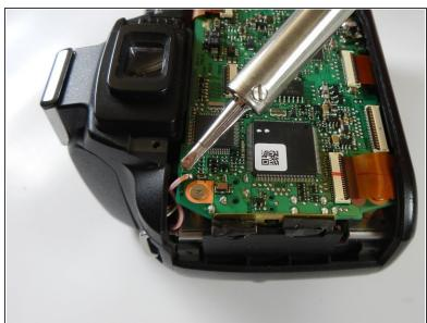
Remove the solder connecting the red wire to the mainboard.
