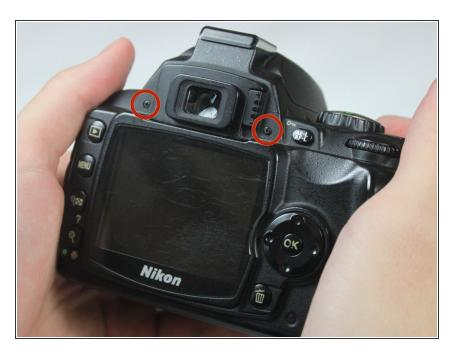
Remove the two visible 6.0 mm
