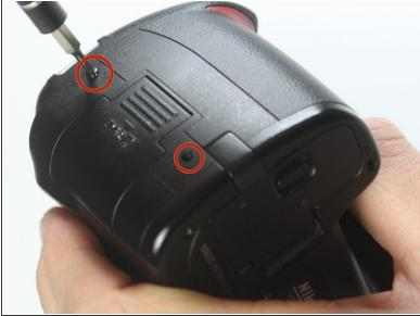
Remove the four 6.0 mm Philips #0 screws on the left and right sides of the camera.
