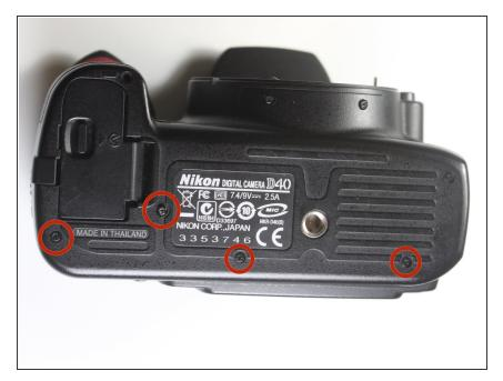
Remove the four highlighted 3.0 mm
