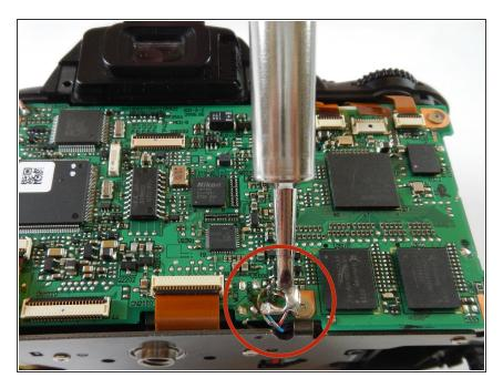
Desolder the 4 smaller wires near the bottom of the mainboard.
