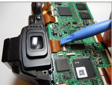
Use the plastic opening tool to release the ribbon cables attached to the mainboard.
