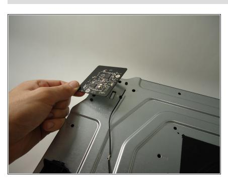
Carefully pull the Wi-Fi board straight up to release it from the chassis. The Wi-Fi board is now free.
