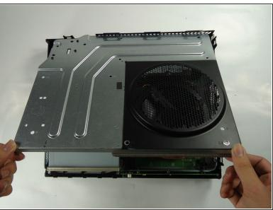
Remove all eight of the 64.0 mm, T-9 screws labeled C1 through C8 securing the chassis top to the motherboard.
