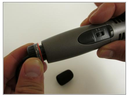
Take off the windshield from the top of the microphone and place aside. The bottom part of the microphone is detachable. In a clockwise motion, begin unscrewing the bottom of the microphone from its base.
