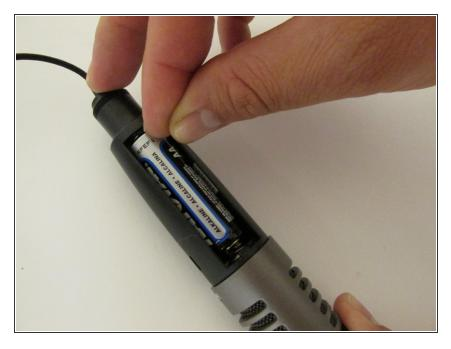
To remove the battery, push it upward into the aluminum spring. This will loosen and free the battery.
