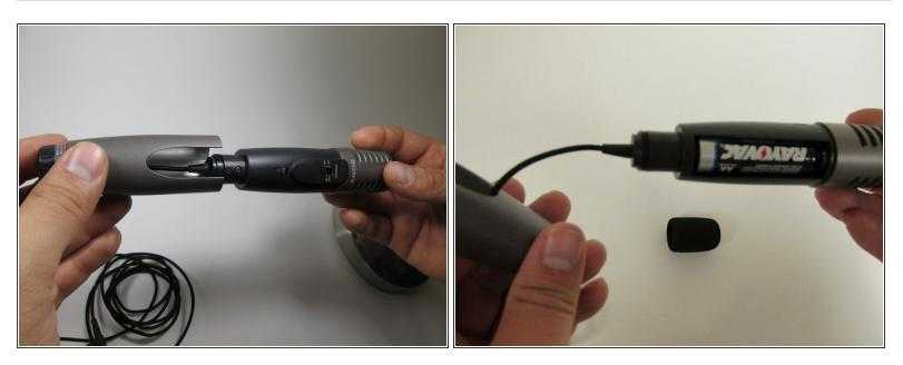
• Pull off the bottom base of the microphone. The microphone should now be in two pieces. After the bottom base is removed, the battery should now be visible.
