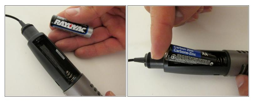
• Select a new, (AA) battery to insert into the microphone. Match the (+) and (-) sides of the battery to the matching symbols inside the microphone.
