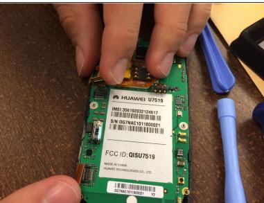
To remove front encasing from the motherboard, first pull back the orange tabs.
