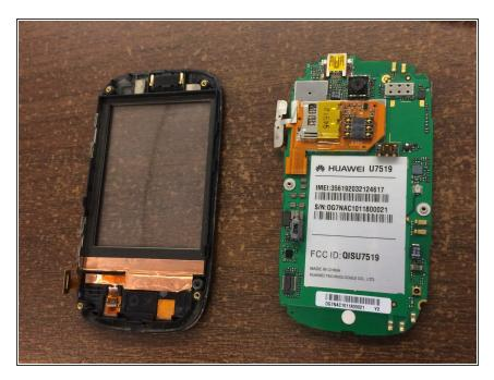
The camera is not removable from the motherboard. Therefore, a new motherboard must be purchased in order to replace the camera.
