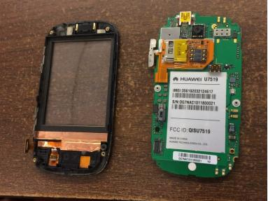
• Once the orange tabs are pulled back, carefully pull the motherboard apart from the front casing.
