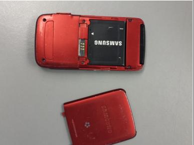
Remove the battery cover by sliding the back panel up. This will expose the battery.
