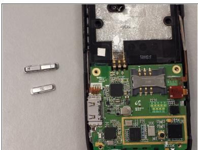
Remove the buttons for the camera and volume.
