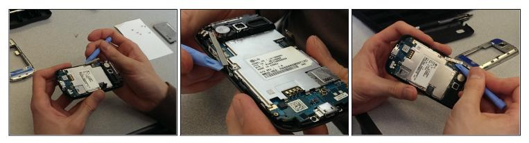
• Pull the volume button away from the case and set aside. It is located on the left side of the phone, and is held to the frame by a small nub.
