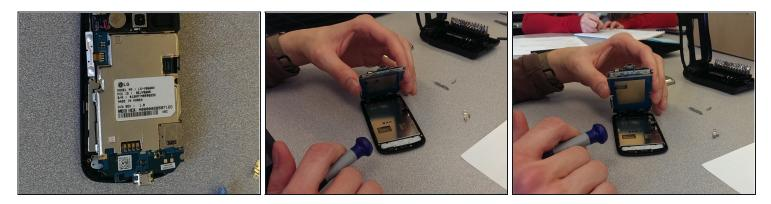
• Lift the system board up and away from the front screen
