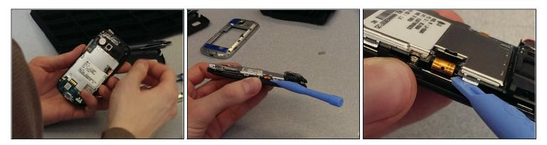
• Unclip the screen connector that is connecting the screen to the system board. It is on the right side of the phone, and looks like a thin piece of bronze plastic.
