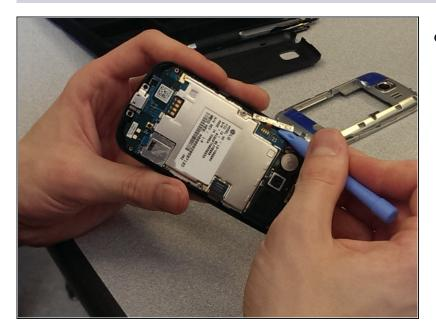
• Pull the white piece underneath the volume button away from the frame.
