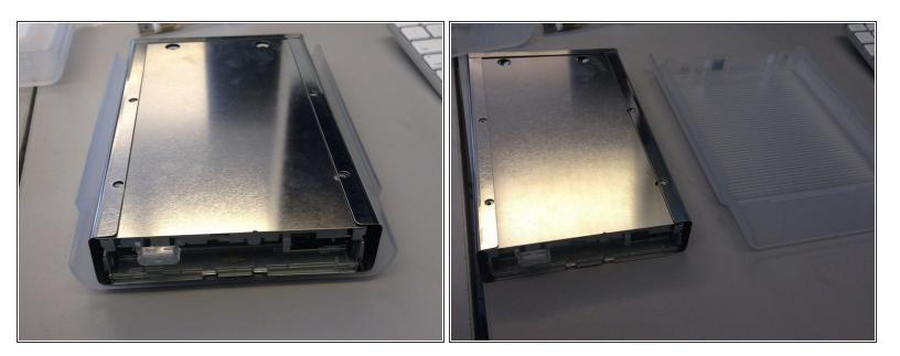
• Slide the metal housing out of the plastic shell.
