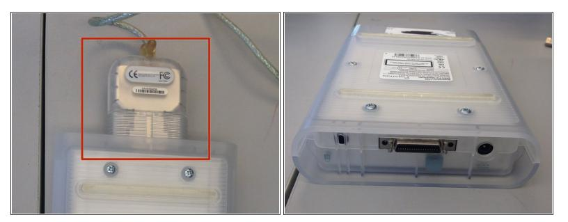
• Remove the USB converter device by gently pulling it out.
