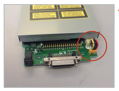
Flip the disk drive over so the the plug on the daughter board is visible.
