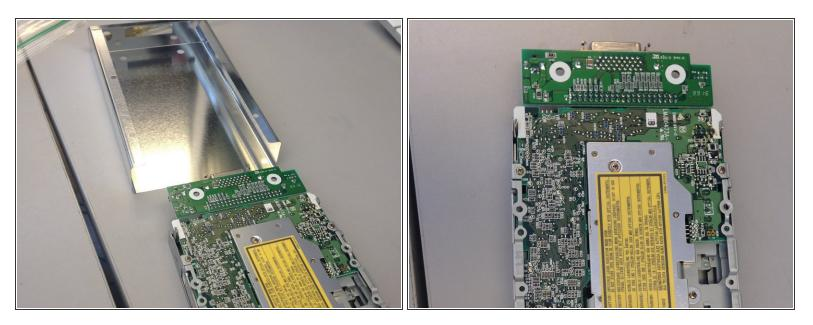
• Slide disk drive out of metal casing.
