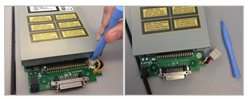
Using an iPod opener put pressure on the white plug and pull backwards until the daughter board unplugs from the main unit.
