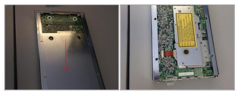
• Slide metal panel out of the metal casing.
