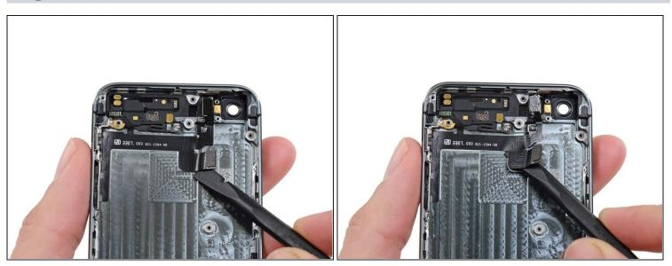
• Slide the flat end of a spudger under the upper component assembly cable to free it from the rear case.
