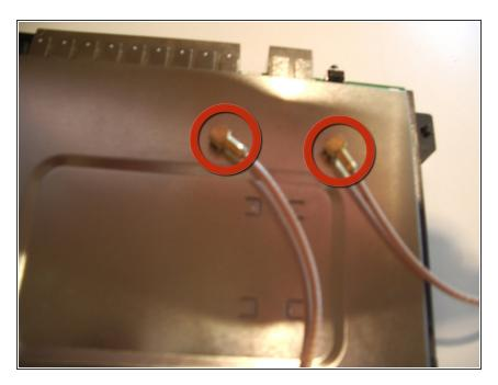
Twist and pull out antenna connector feeds.
