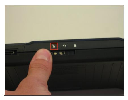
Slide the tab located at the top of the calculator to the unlocked position.
