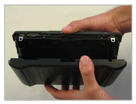
Slide the back cover down, and then pull the back plate away from the calculator.
