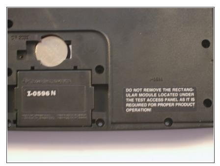
The warning label next to this module reads "Do not remove the rectangular module located under the test access panel as it is required for proper product operation!"
