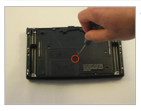
Unscrew the back-up battery cover. (1 screw)
