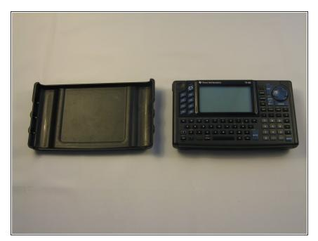
Remove the protective cover. This will easily unsnap from the main body.
