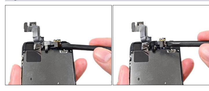
• Use the flat end of a spudger to gently peel the front-facing camera portion of the cable away from the display assembly.
