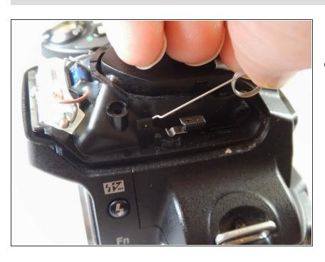
Remove metal spring and replace with new spring. To reassemble your device, follow these instructions in reverse order.
