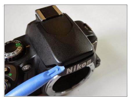
Pry the flash open using the plastic opening tool.
