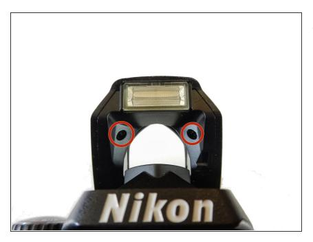
Remove the two Phillips #0 3.0 mm screws from the front of the flash compartment using the small Phillips Head screwdriver.
