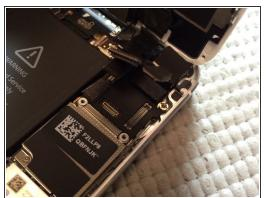
Remove four screws from shield covering display assembly connectors. Lift connectors using nylon spudger.
