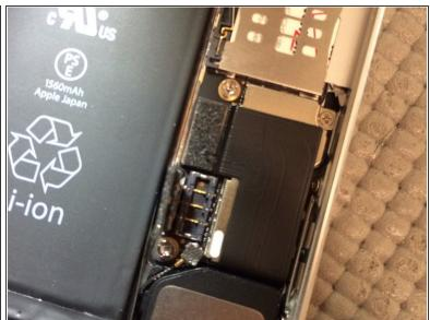
Disconnect battery before screen removal by removing 2 screws from shield. Once shield is removed, disconnect battery using nylon spudger. (DO NOT USE METAL TOOLS)
