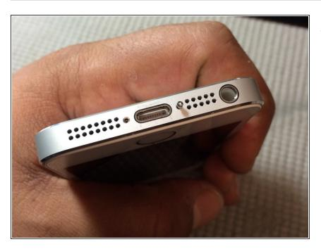
Remove pentalobe screws with torx screwdriver.
