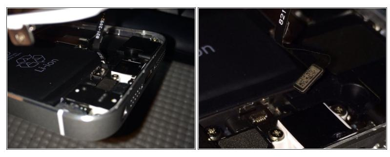
After using spudger or suction cup to lift screen. Be careful not to pull screen completely up. The touch id sensor flex cable is attached near the home button. There is a small metal clip that needs to be carefully pry'd off before removing flex cable connector.
