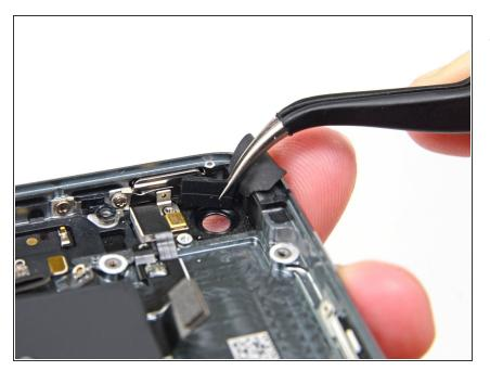
• Remove the rubber camera bumper from the case.
