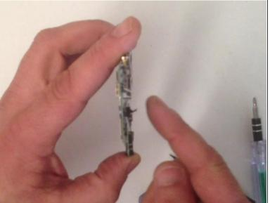
I used soldering station to remove the old one and put the new one (UMD switch).
