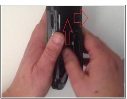
Unhook the door metal plate and disassemble UMD door.
