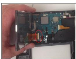
Disconnect and remove the display.
