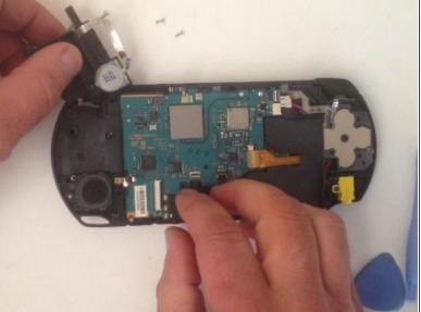
I must disconnect 7x cables and unscrew a screw.
