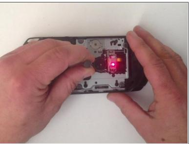
With a screwdriver I short the UMD switch to test the laser.
