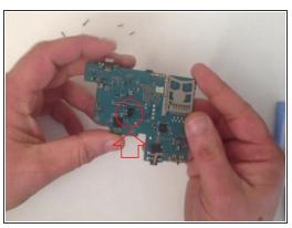
Now I disconnect the battery connector and here is the mainboard.
