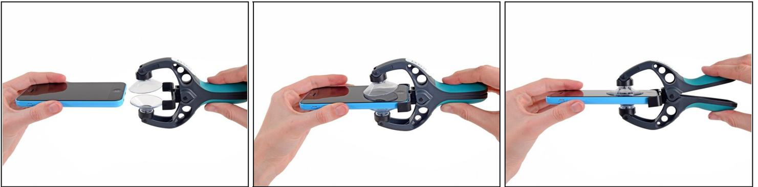
ⓘ The next two steps demonstrate using the [iSlack](#), a great tool for safely opening the iPhone 5c that we recommend for anyone doing more than one repair on an iPhone 5, 5s, or 5c. **If you aren't using the iSlack, skip to [Step 5](#).**
