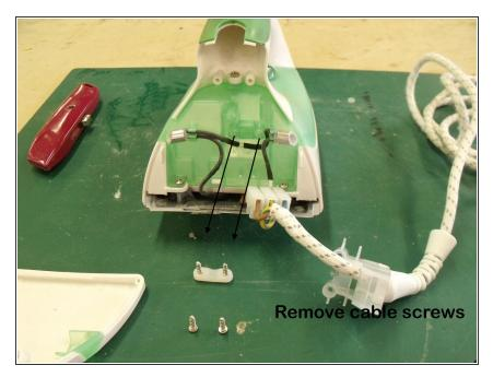
Next remove the cable bridge bracket.
