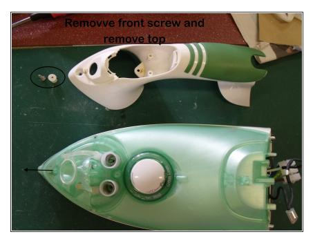
Remove front of the iron by undoing the screw (arrow) by first taking off cover cap.
