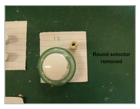
Next take out round selector, this is simply clipped so can be pulled out with pliers.
