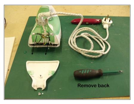
• First remove the rear or the iron using the flathead screwdriver.
