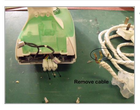
To free the long cable remove from terminal block at rear.
