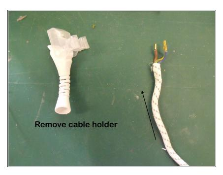
slide off the cable holder from the cable.
