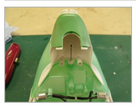
Next remove the screw the hold the top on.
