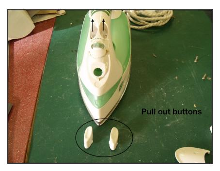
At the front of the iron pull out the buttons for the steam and water.
