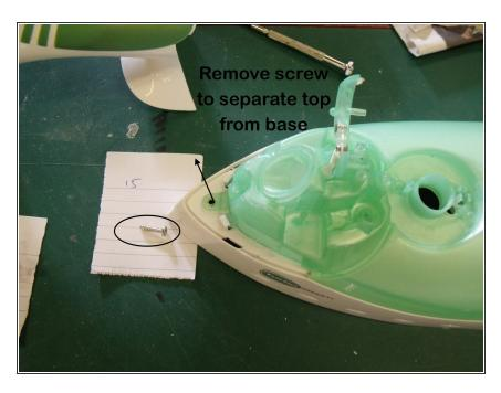
Remove the screw (circled) this will lead to the separation of the base and the top.
