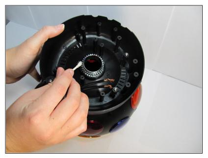
Apply oil to the gear directly from the oil bottle or with a Qtip.
