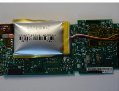
3. Carefully remove the connected wires underneath the motherboard to disconnect the clickwheel and the screen.
