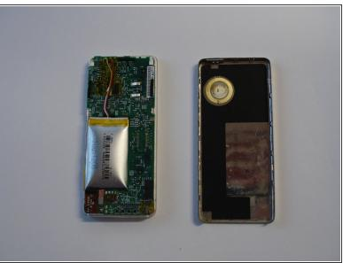
• 1. Using an ipod unclipping tool (which could be a knife or similar to it), unclip the outer casing by putting the tool up to the connection point. This should pop the case off. Note that force will need to be used.
