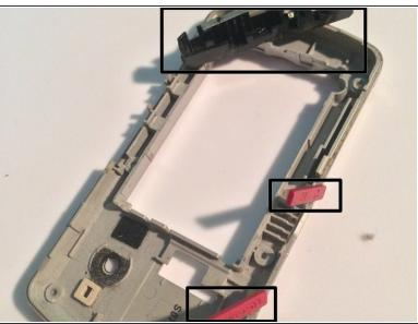
It is possible to remove and swap out these parts before reassembly: battery cover release button, grounding clip, charging and SD card slot covers, plastic/metal framework
